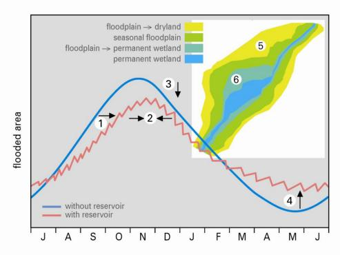
Fig. 3.3. Dams in river basins in (semi)arid climates as in the Sahel have in general six main effects: 1) the timing of the flood will be retarded, 2) the flood peak will be smaller, 3) the flood peak will be lowered, 4) the river discharge during the dry period will be increased, 5) floodplains will be reduced in favour of drylands, 6) permanent wetlands infested by invasive plant, mainly Typha, will increase (from Zwarts et al. 2009).
