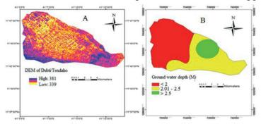
Figure 4. 5: (A) Digital elevation model in meters above sea level and (B) groundwater depth and its spatial extent at Dubti/Tendaho state farm (Shimellis Abdi Assefa, 2016)
